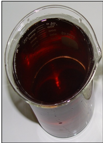
Raw Water 498(CU)
